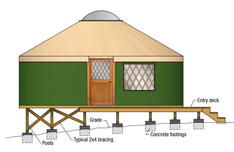
Note: Platform and footings should be designed according to the conditions of each individual site and local building requirements. Site and soil conditions will dictate footing size and depth below grade.
