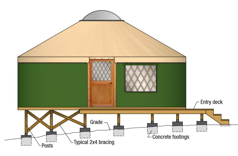
Note: Platform and footings should be designed according to the conditions of each individual site and local building requirements. Site and soil conditions will dictate footing size and depth below grade.
