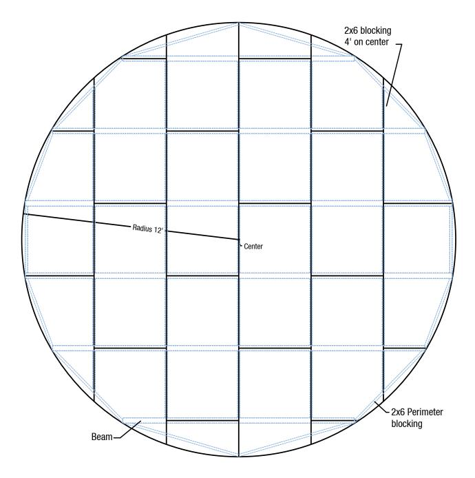
**1.)** Make a compass using a board or non-stretch string and a nail at the center to mark radius.
